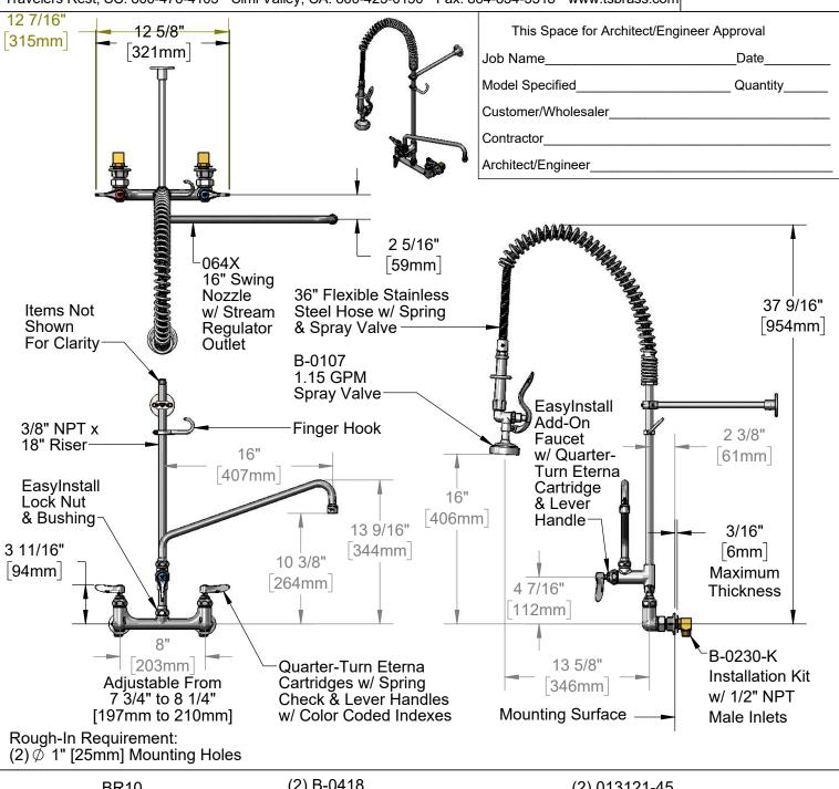
BR10 Brush Attachment for B-0107 Spray Valve (Included) (2) B-0418 1/2" NPT Female Inlet Supply Stop (Included)
