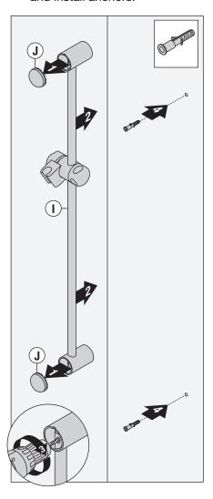
**Notes:** Make sure that 30" slide bar holes and bracket holes are aligned before drilling. Before drilling bottom hole, make sure 30" slide bar is plumb.
