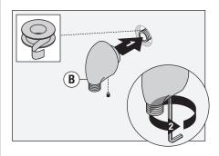
10) Attach large end of hand shower hose (A) to hand shower head (H). Attach small end of hand shower hose (A) to wall elbow (B). Turn clockwise to tighten.
