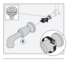
8) Install wall cradle (A) to pipe fitting. Turn clockwise to tighten.
