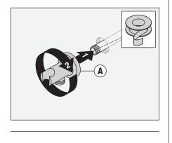
9) Attach shower arm (B) to vertical shower pipe. Turn clockwise to tighten.
