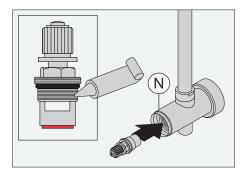
**Installation Tip:** Back off cartridge slightly to ensure proper handle alignment if necessary.
