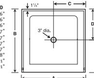
IMPORTANT: Rough-in dimensions are provided for reference only. You must measure the actual shower pan and check local building code requirements before construction of the stud wall.
