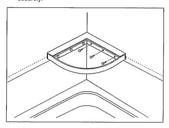
The locking tabs on the underside of the Swanstone seat must engage behind the stainless steel bracket to prevent the seat from moving away from the wall. Do not apply silicone until you have trial fit the seat and made sure the locking tabs fully engage. Failure to follow this procedure may result in serious injury.
