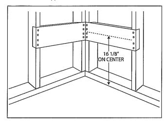
NOTE: After installing the 2  $\times$  6 wall support, finish out the wall with drywall and a Swanstone wall panel system or a wall covering of your choice. After the wall covering has been installed, set, and allowed to cure, move on to Step 3.
