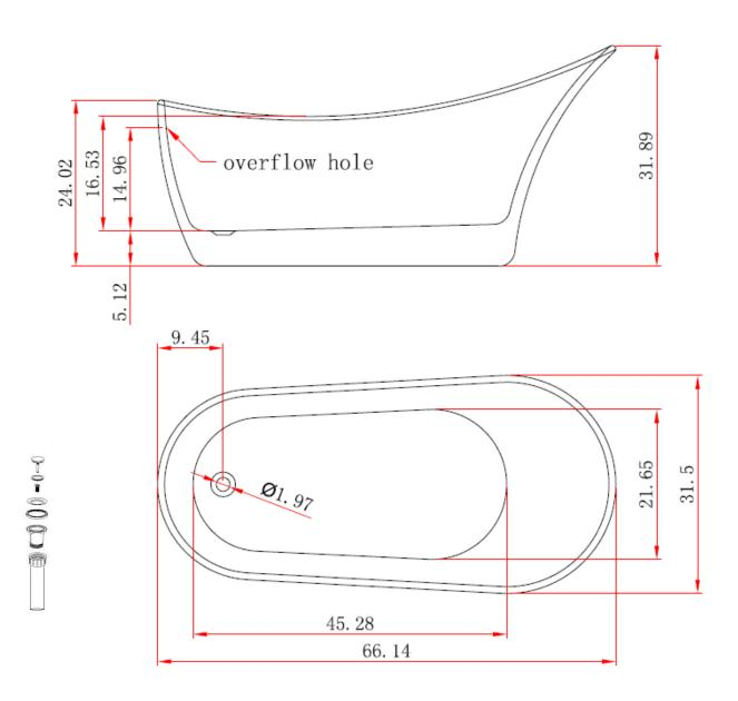
The Overflow channel is molded into the interior tub wall. Drain is included. Please use a bead of silicone around the base of the tub to provide a seal between the tub and the floor, and to prevent the tub from moving.
