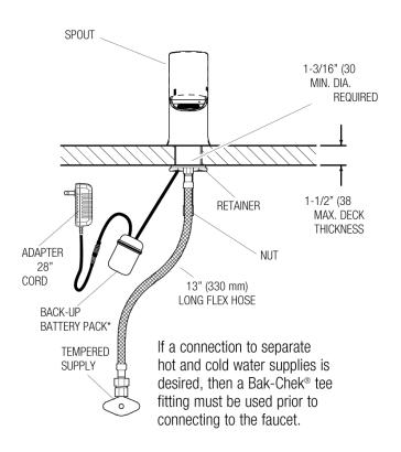
1070 requirements. The product shall be tested and certified to industry standards: ASME A112.18.1M, CSAB125.1, California Health and Safety Code 116875 (AB1953-2006), and Vermont Bill S.152. This product meets ADA ANSI/ICC A117.1requirements.
