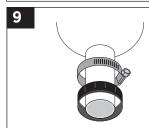
PLACE THE GEAR CLAMP and compression nut onto the housing tailpipe.
