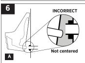
A. Hang the bowl on the bracket and check tall pipe alignment, then remove the bowl and adjust the bracket as needed. Re-hang and re-check bowl alignment with drain line. Tail pipe should align with center or
