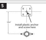
MEASURE & MARK THE ROUGH-IN If in-wall carrier is not used. Use a 5/16" masonry bit to drill hole, then install the hanger bracket with one plastic anchor and screw.
