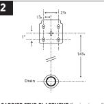
**CARRIER STUD PLACEMENT** If using in-wall carrier, set bearing as shown above.
