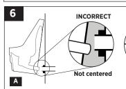
A. Hang the bowl on the bracket and check tall pipe alignment, then remove the bowl and adjust the bracket as needed.
