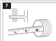
**DETERMINE THE DRAIN NIPPLE DEPTH** by measuring the distance between the back of the sanitary tee (or elbow) to the front edge of the nipple.
