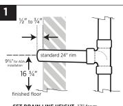
SET DRAIN LINE HEIGHT 17" from finished floor (standard 24" rim) or 10" for ADA installation. Threaded nipple should extend ½ to ¾" from wall.
