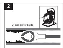
IMPORTANT: Use a drain machine to remove build-up inside pipes. Clean up to 25 feet deep then finish with water to remove cutting debris.
