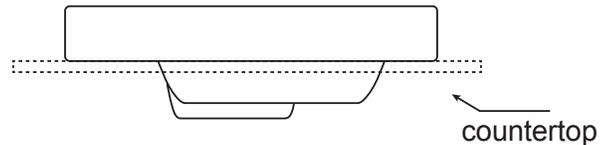
**Step 3 :** Place a generous portion of plumbers' putty under drain cap and insert whole drain body inside the bowl and through the countertop.
