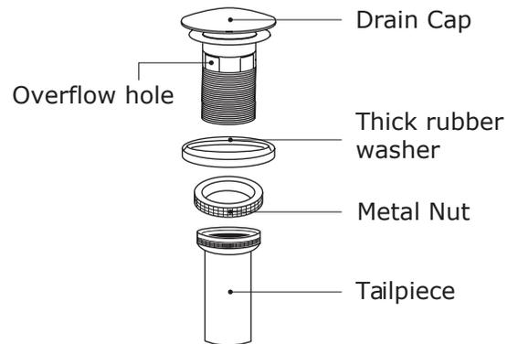
**Step 4 :** From under the drain, insert the thick rubber washer and screw on and tighten the metal nut. Remove excess plumbers' putty
