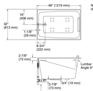
2-5/8" (67 mm) No change in measurement if connected with drain illustrated. (K-7265)
