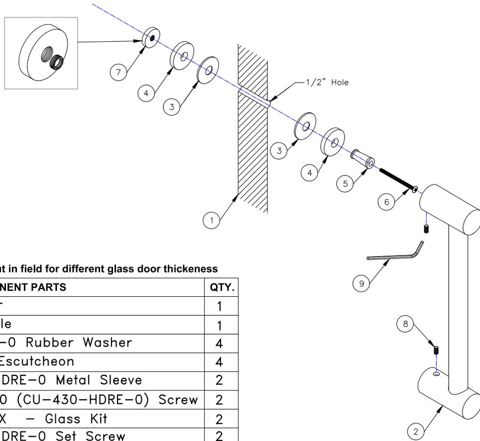
\*Screw is able to be cut in field for different glass door thickness
