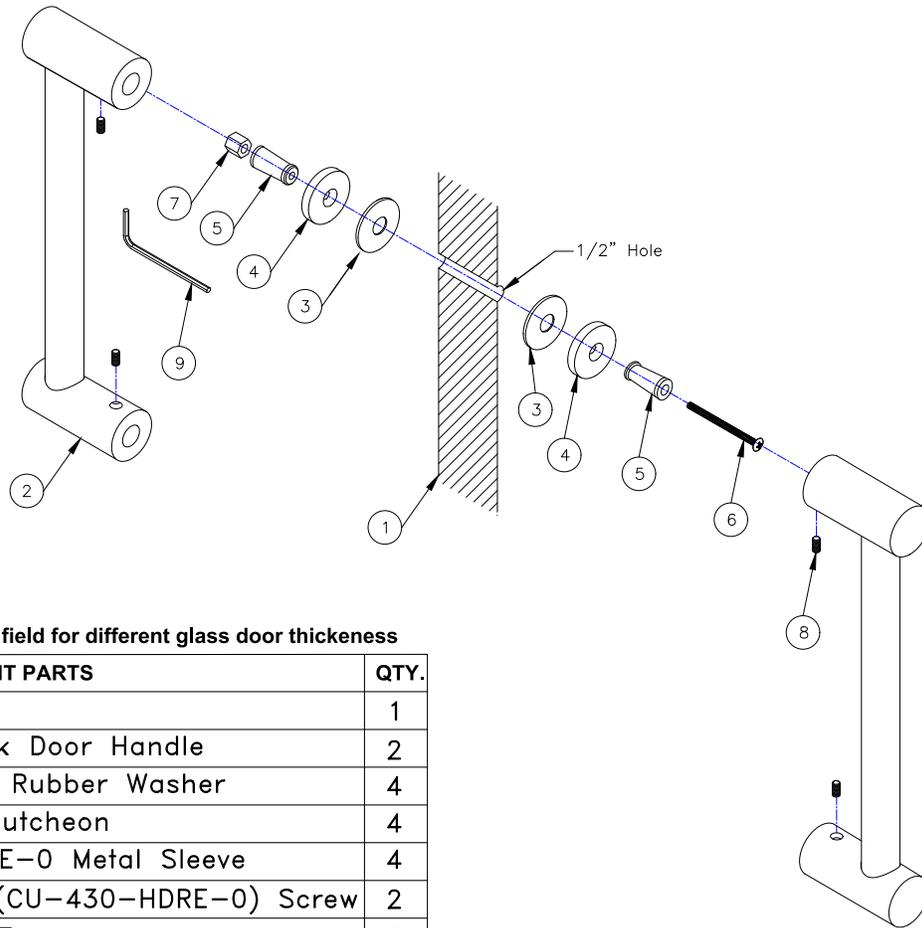
\*Screw is able to be cut in field for different glass door thickness
