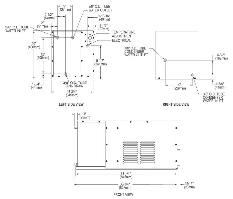
**NOTE:** This unit is intended for remote installation only. It is important to insure proper ventilation. Allow a minimum clearance of 6"(152mm) in front and 6"(152mm) in the rear of unit.
