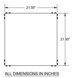
The QUICKSTAND™ #40-S-22- (A or U) stands safely elevates water heaters and other equipment above the floor (900 lbs rating).
