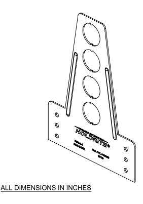
The LOCKRITE<sup>™</sup> #609-N-6 is a 16 gage galvanized steel bracket with 1" hole on 1-1/4" centers. Ideal for toilets or hose bib stub-outs. Also serves as a nail plate. This bracket is designed to work exclusively with our glueable HOLDRITE<sup>®</sup> #604 (1/2") of #605 (3/4") inserts when installing CPVC tubing. Inserts snaps into bracket.
