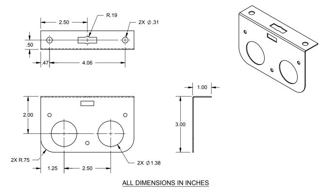
The HOLDRITE® #121-D is a 20 gage galvanized steel bracket that supports dual lines of 1/2", 3/4" or 1" Copper, PEX or CPVC tubing at 2" center line height. The hole pattern on the 90° base allows for attachment to any flat surface. The bracket can also be suspended by 3/8" threaded rod.
