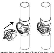
Insert Test Wedge into Clean Out Tee, with "pressure side" up. (Prior to installation, be sure all contact surfaces are clean and free of excess glue, etc.)
