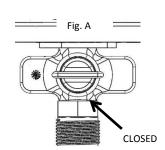
If using Test Wedge with valve stem, turn spigot ball valve to the "closed" position (See Fig A). Fill pipe stack (maximum 50' head/22PSI).
