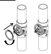
Re-install Spanner Ring onto Clean Out Tee. Tighten completely (utilize spanner wrench).
