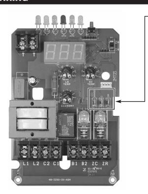
Locate the three quick connect posts on the HydroStat circuit board. The sensor cable will plug into two of these terminals depending on the features to be used.
