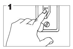
WARNING - To prevent electrical shock or equipment damage, power must be off during installation or servicing of the control. To prevent serious burns, the boiler should be thoroughly cooled before installing or servicing control. Only qualified personnel may install or service the control in accordance with local codes and ordinances. Read instructions completely before proceeding.
