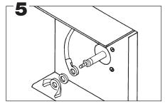
Connect the ring terminal wire lead to the probe terminal stud and secure with the lock washer and wing nut provided. With the power removed, proceed with installation and wiring according to the instructions on page 2. Upon completion of wiring replace control cover.
