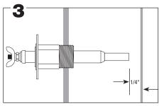
Allow 1/4" clearance from the probe to any boiler surface, tube or baffle. NOTE: Excessive use of Teflon tape to seal probe piping threads may insulate the control from boiler ground. This could result in the control not operating.
