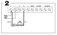
Connect terminal 2 to burner circuit neutral.
