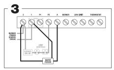
Optional water feeder connection. Connect feeder N to terminal 2. Connect Feeder H to terminal 1. Connect feeder "FEED" or "W" to terminal A. For water feeders with 2 leads, connect feeder neutral to terminal 2 and feeder hot to terminal A. Note: Use of a solenoid valve or McDonnell & Miller Model 101A water feeder may cause flooding and is not recommended for use with this low water
