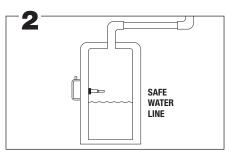
The probe may be installed in the boiler above the lowest safe water level established by the boiler manufacturer. Most manufacturers provide a suitable opening in the side of the boiler.
