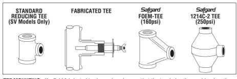
**TEE MOUNTING:** If a field fabricated tee is used, make sure that the tee drains thoroughly when the water level falls below it, and that it conforms to the spacing requirements described in Step 3. Models equipped with the shorter EL1214-SV probe can be installed in most standard reducing tees. Safgard cast iron tees are also available to accommodate all probe models (See page 4).
