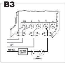
Connect terminal P2 to burner circuit in series with and before other limit controls.
