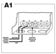
Connect the hot lead of the input voltage (120 VAC, 60 HZ) to terminal H. Connect the neutral lead to terminal GN.
