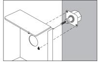
Slide keyhole slots over probe mounting screws and tighten screws (with either a 1/4" hex head driver or flat screwdriver).
