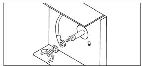
Connect the ring terminal wire lead to the probe terminal stud and secure with the lock washer and wing nut provided. *With the power removed*, proceed with installation and wiring according to Method A or B described on next page.
