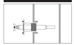
Check to insure 1/4" clearance from probe to any surface within the boiler or tee. When installed in a tee, the probe tip should extend fully into the pipe run. Apply pipe sealing compound to threads.
