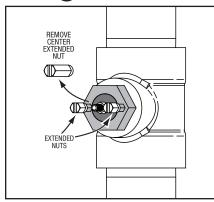
Remove center extended nut. Apply pipe sealing compound to probe threads and install in boiler or tee (Teflon tape is not recommended). Tighten so that the two smaller extended nuts are horizontally aligned.
