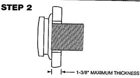
Place push button assembly in 1-1/2" hole. Tighten with hardware.
