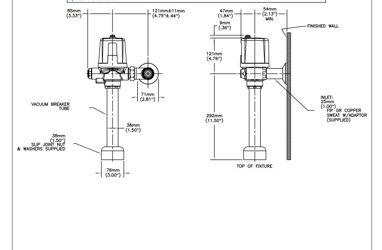
Delta reserves the right (1) to make changes to specifications and materials, and (2) to change or discontinue models, both without notice or obligation. Dimensions are for reference. Measurement may vary plus or minus 6mm(0.25"). Mounting locations are suggested only. Check with local codes for requirements in your area. This spec was produced April 14, 2021.
