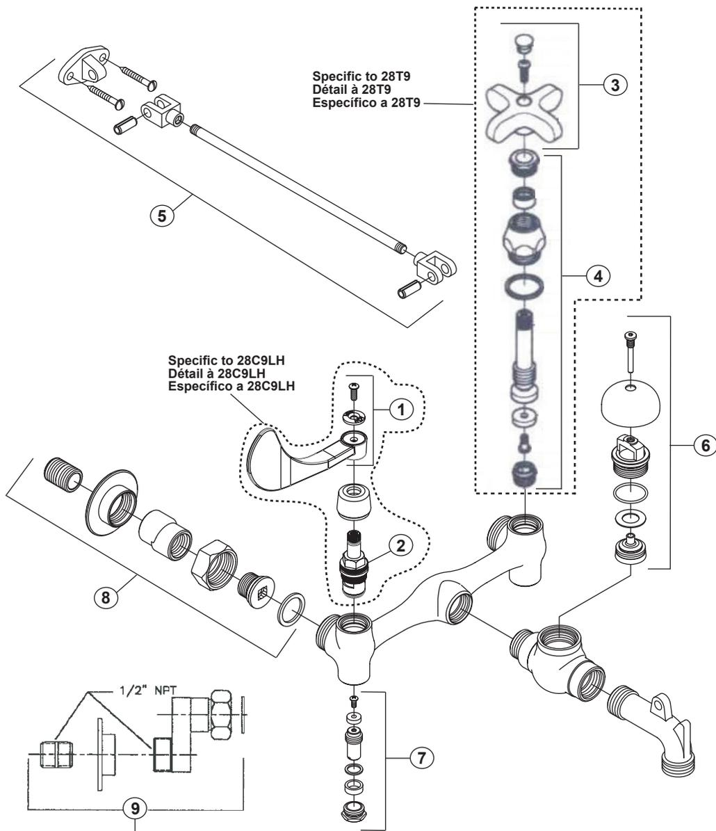
**NOTE:** Cartridges are not interchangeable as the bodies between the "T" & "C" series are machined differently.
