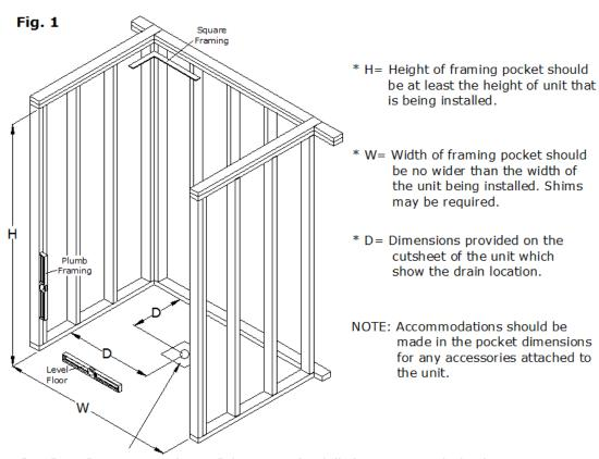
$8" \times 8"$  or 8" Dia. Core at least 2" deep must be drilled on center with the drain to permit the drain area to be pulled down by the plumbing connection. The drain must be aligned in the center of the core to insure proper installation and drainage slope.
