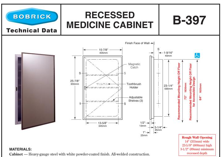
**Door** — Heavy-gauge steel with stainless steel channel frame. Secured to cabinet with an enameled steel piano-hinge and equipped with a magnetic catch. Furnished with toothbrush holder that mounts on back of door.
