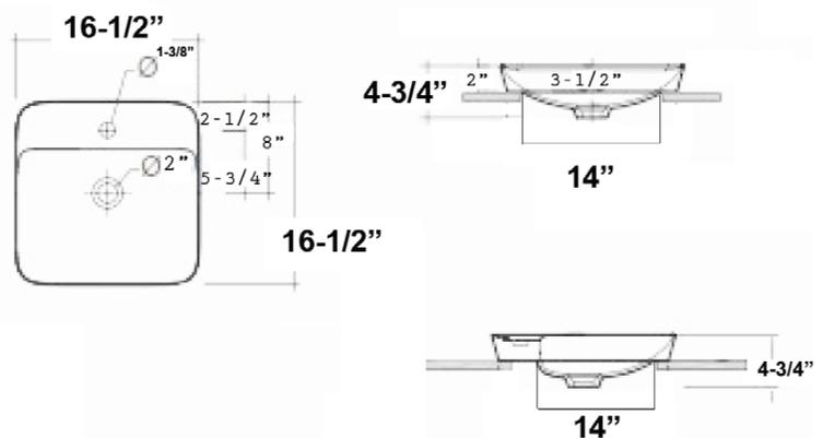
Dimensions of fixture are nominal and may vary within the range of tolerances established by ASME Standard A112.19.2.2018 Dimensions and specifications subject to change without notice.
