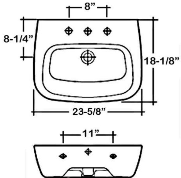
Dimensions of fixture are nominal and may vary within the range of tolerances established by ASME Standard A112.19.2.2018. Dimensions and specifications subject to change without notice.
