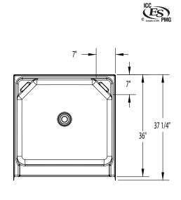
FEATURES Ibs Dimensional Tolerance ± %". Dimensions needed for site preparation should be measured from the unit. Aquatic assumes no responsibility for preparatory work.
