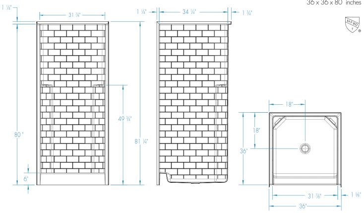
$\label{eq:FEATURES} \textbf{ Dimensional Tolerance} \pm \textbf{\%}''. \textbf{ Dimensions needed for site preparation should be measured from the unit. Aquatic assumes no responsibility for preparatory work.}$
